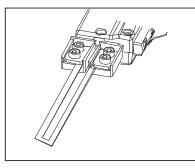
*NOTE:* Always unpress the trigger of the *DC180E* Hot Knife before installing or removing the blades. Allow sufficient cooling time for blades, blade holders and mounting crews before handing.
